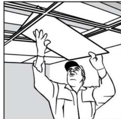
4. Placing the tiles in the grid frames
